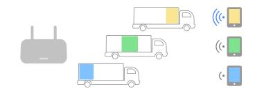
More Devices: Wi-Fi 6 uses OFDMA to improve capacity and efficiency of your network, so more devices can connect without slowing down your Wi-Fi.
