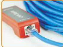
Verify Lan Cable Condition
