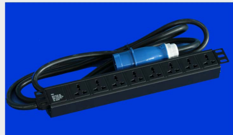
8-outlet All-usage PDU, 2P+E industrial plug 32A input, 10A all usage outlet, without switch, with 3.0m length cable, 19" positive installation with TOTEN logo (322000796)
