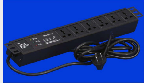
6-outlet All-usage PDU, 10A input and output, with lighting protection and without switch, 3.0m length cable, 19" positive installation, with TOTEN logo (PD.0601.9100)
