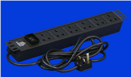
6-outlet UK-type PDU, 13A input and output, with master switch, 3.0m length cable, 19" positive installation with TOTEN logo (PD.0602.9000)
