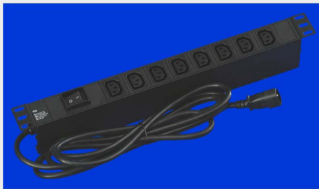
8-outlet PDU, IEC320 C14 plug 10A input, EC320 C13 outlet 10A output, with masterswitch, 3.0m length cable, 19" positive installation with TOTEN logo (322000742)
